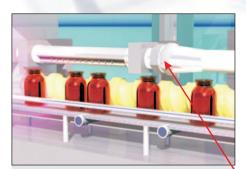
The autoclavable HAUG ionizing bar "EI VAC" ... unique. It is mounted here transverse across a screw conveyor for the electrostatic discharge of the upper area of a bottleneck before filling.
